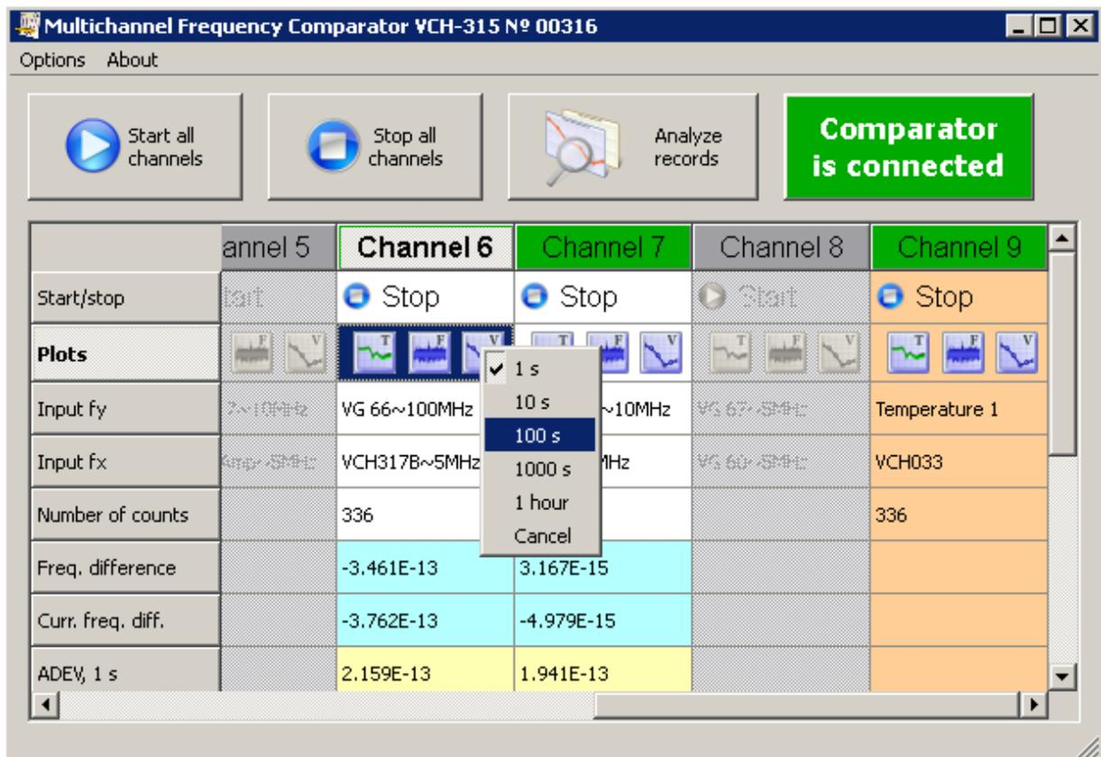
**Figure 6.3** – Main window. Selecting averaging interval for the phase and frequency graphs
