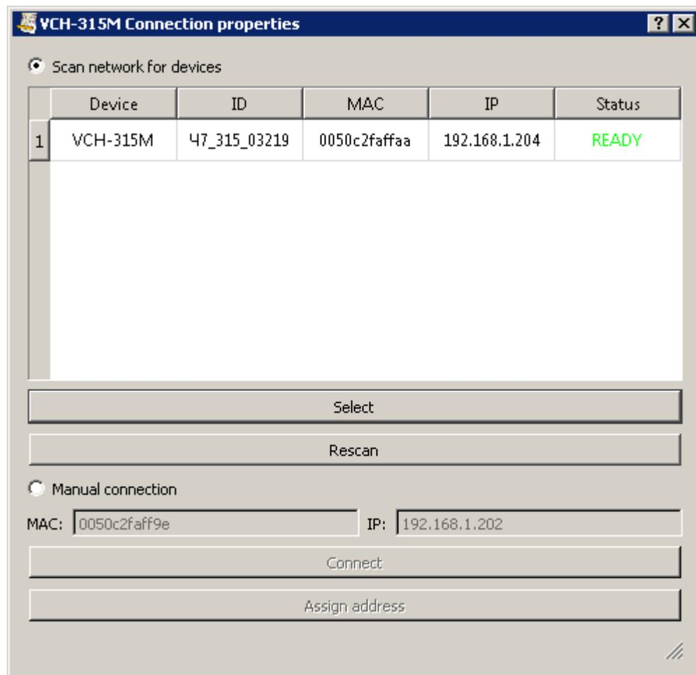
**Figure 5.2** – Window "Connection properties"
