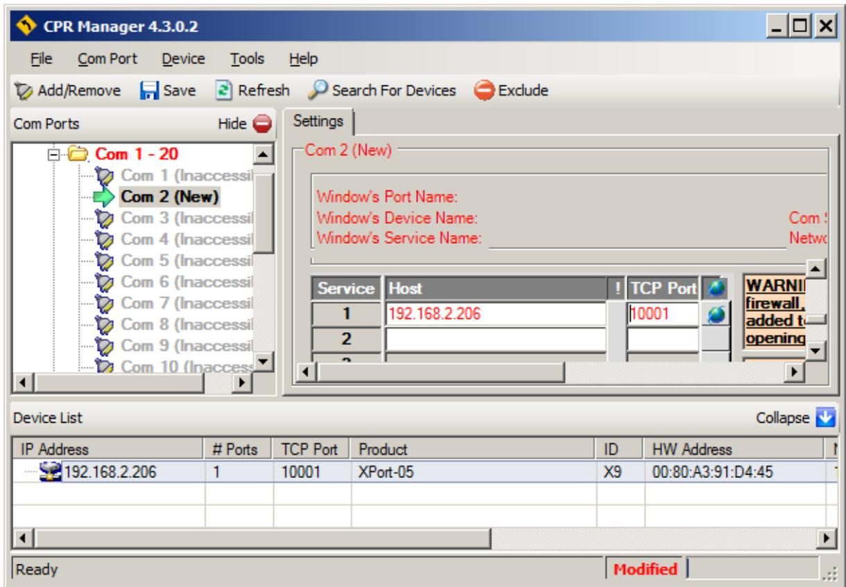
**Figure 4.4** – Selecting device from the list by its MAC-address (only one device shown here)
