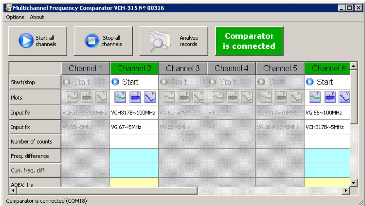
**Figure 5.5** – Main window after connection is established
