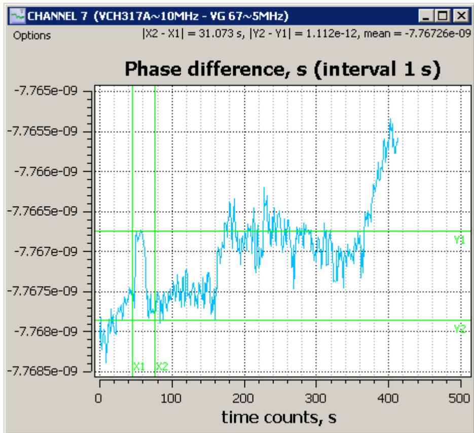
**Figure 6.4** – Phase difference graph for averaging interval of 1 s
