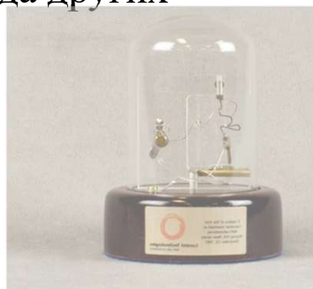
Replica of First Transistor Invented at Bell Labs December 23, 1947
