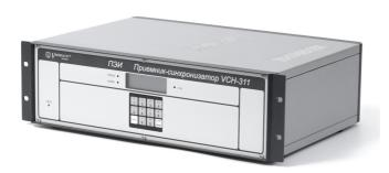
GPS/GLONASS disciplined rubidium frequency standard model VCH-311 contains multi-channel GPS/GLONASS receiver, time scale comparison unit and automatically adjustable Rubidium reference oscillator. The instrument is intended to use as a high stable frequency signal source (STANDARD mode), or precision frequency calibrator for any external standard signals (CALIBRATOR mode).
