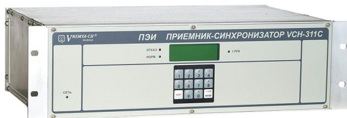
GPS/GLONASS primary reference source VCH-311C contains multi-channel GPS/GLONASS receiver, time scale comparison unit and automatically adjustable Rubidium reference oscillator.
