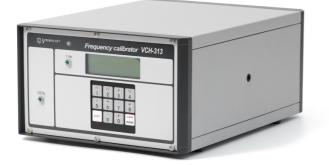
Frequency calibrator VCH-313 is intended for calibration and verification of different frequency signal sources, using precision time scale signal, transmitted by satellite navigation systems GPS/GLONASS. The instrument can provides periodical frequency correction of the calibrating frequency standard in automatic mode.
