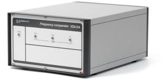
Frequency comparator VCH-314 is intended for precise phase and frequency instability measurements. It contains two identical measuring channels (four input signals). Using crosscorrelation technique in allows to obtain super-low measurement error and to calculate frequency instability of each single signal separately.
