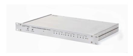
Frequency distribution amplifier is designed for ultralow-noise distribution of sinusoidal signals 1-100 MHz with unity gain. It allows checking for signals availability via RS-232 interface. The basic model has 3 inputs / 12 outputs (3 modules 1 / 4). For the information about possible
